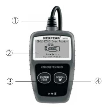
**OBDII CONNECTOR** - Connects the scan tool to the vehicle's Data Link Connector (DLC).
